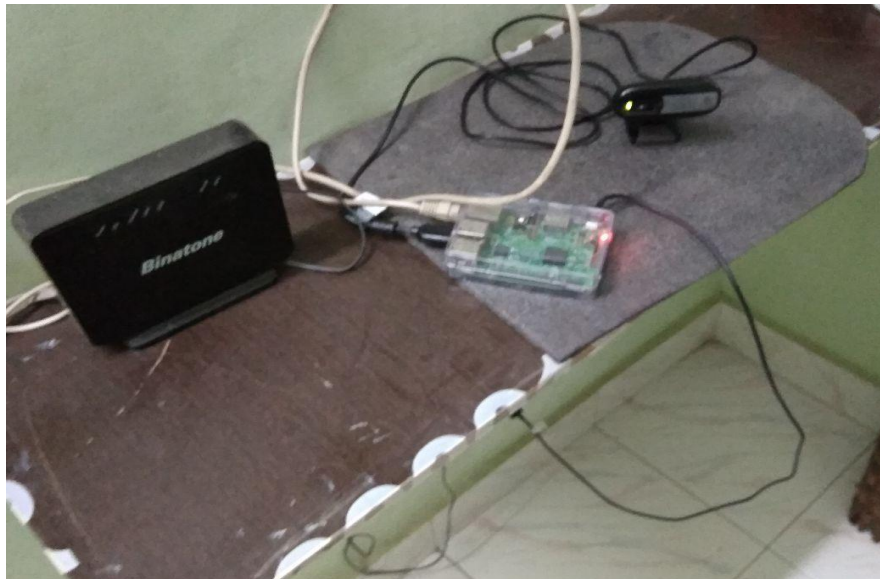
Fig.2. Raspberry Pi accessing the router to act as a server for the Android app
