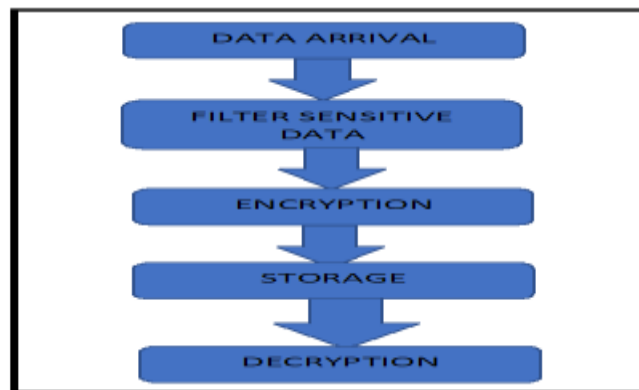
Fig 2: Encryption process after applying filtering method based on criteria set.
